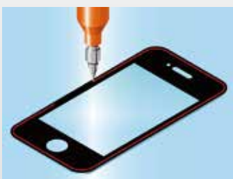
Sealant dispensing of PUR for smartphone's cover
