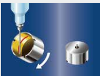
Dispensing of 2-part epoxy adhesive to motors
