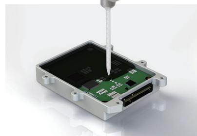
Potting of onboard vehicle substrates
