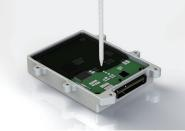
Potting of onboard vehicle substrates
