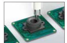
UV dispensing for fixing the automotive camera lens.
