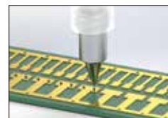
Solder paste dispensing to lead frame
