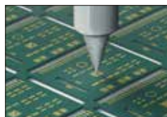
Ag paste dispensing for die bonding
