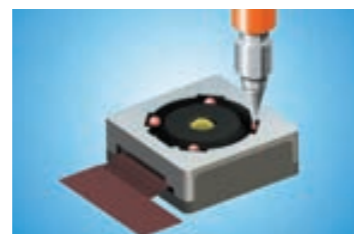
UV dispensing on camera modules
