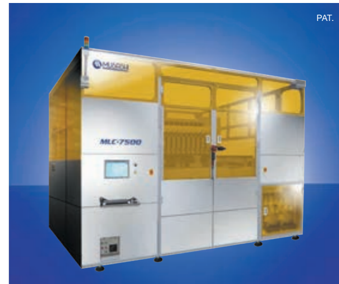
Fully automated ODF machine MLC-7500
