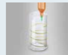
Spiral dispensing onto the inner surface of a cylinder
