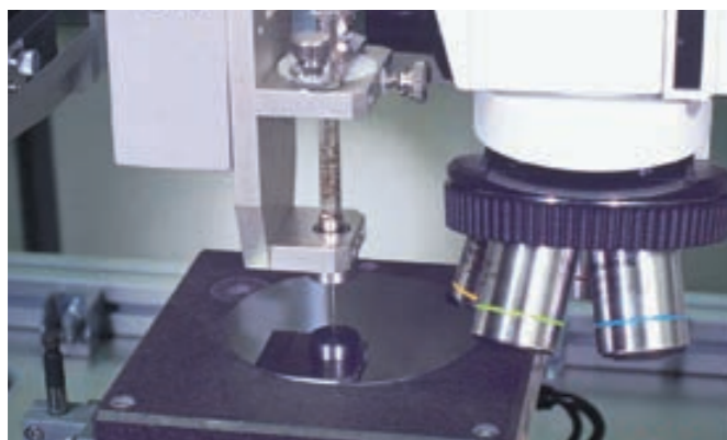
Example of FA dispense machine with micro syringe specifications
