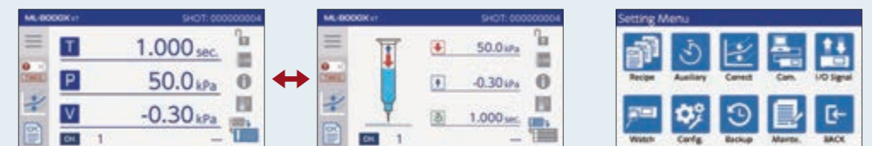
Two types of main screens are available: "Parameter Operation" and "Visual Operation".
