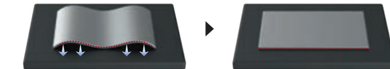
Workpieces are fixed by sucking through stage suction holes.
