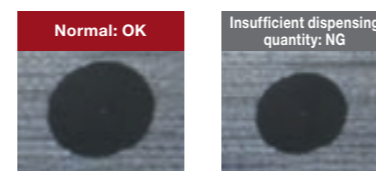
Pattern matching, OK / NG determination based on contact diameter
