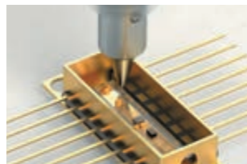
Dispensing Ag Paste on optical communication module
