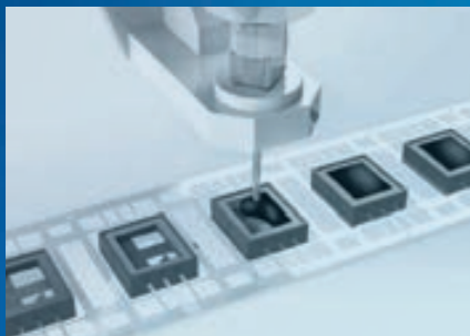
Potting on sensor components
