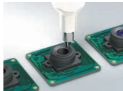
UV dispensing for fixed automotive camera lenses
